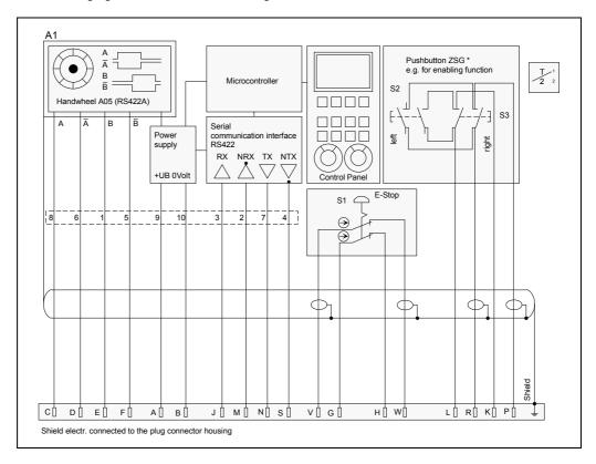
The HBLS handwheel must be connected to the CNC as shown in the next figure.
