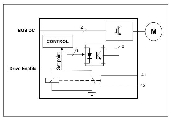
The "Drive Enable" pin already available on conventional Fagor drives works the same way on drives with Safe Disable although it has been implemented keeping the safety principles and protocols in mind.
