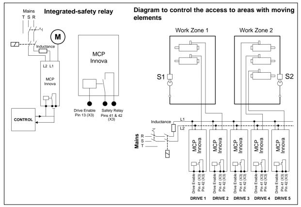
The diagram to control the access to areas with moving elements is:
