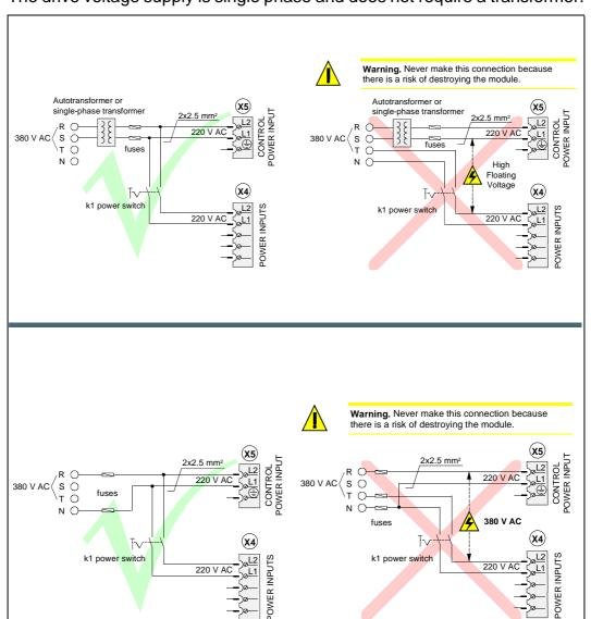
The drive voltage supply is single phase and does not require a transformer.
