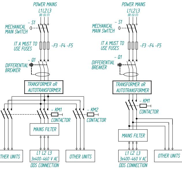
**Note.** The mains filter may be installed indistinctly before or after the power switch -KM1.
