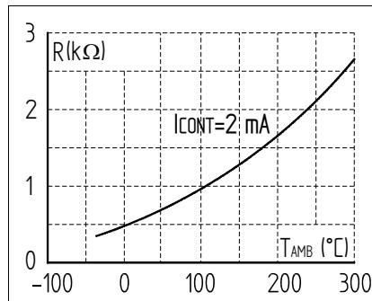
The following figure shows the resistance of the sensor as a function of the ambient temperature (average values).
