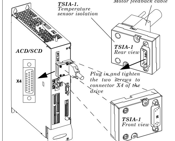
**Note.** The pinout of the temperature sensor isolation adapter TSIA-1 is the same as that of connector X4 of the drive's motor feedback.
