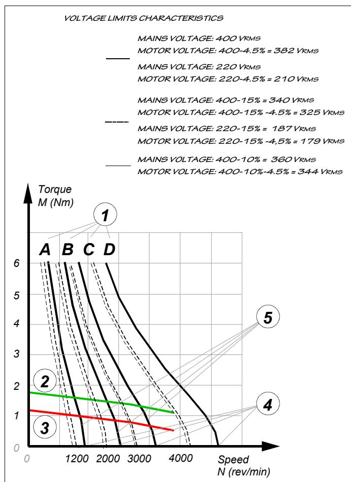
1. Curves for torque limitation by voltage depending on type of stator winding.
