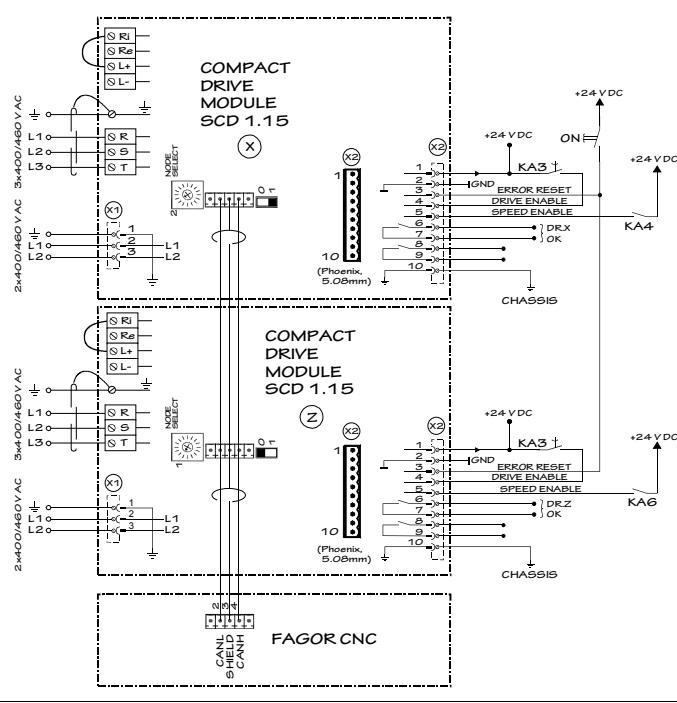
**Note.** The relay -KA3 uses delayed deactivation (t sec.) maintaining the DRIVE ENABLE control signal active for a few seconds to maintain motor torque while the vertical axis holding brake is enabled.
