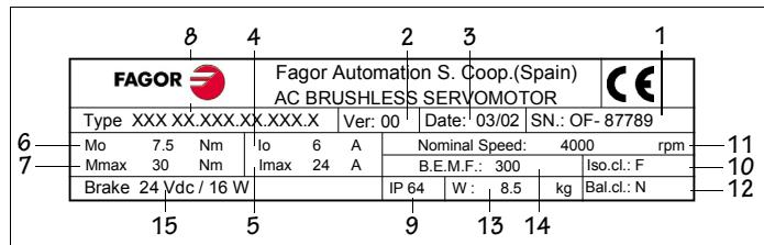
This characteristics plate of the motor is located on the right side of the motor viewed from its shaft. The items shown on this plate are:
