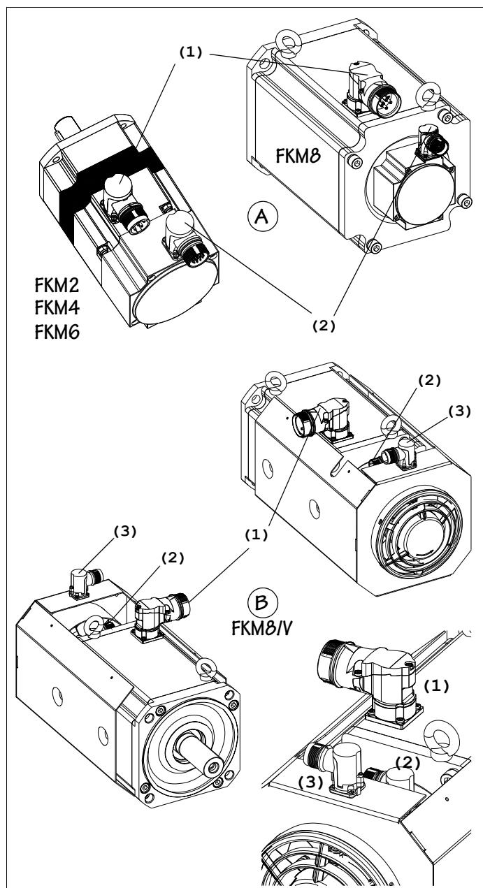
FKM servomotors. A. Without FAN. B. With FAN.
