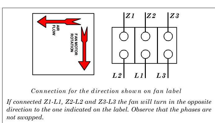
Connection for the direction shown on fan label
