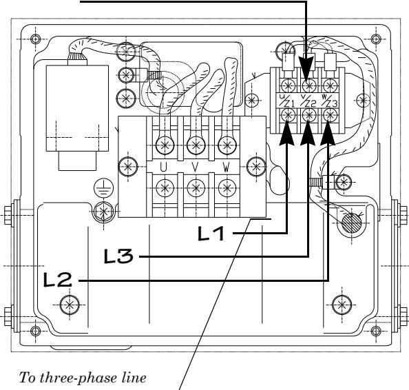
Note that phases L1 and L2 are swapped for proper air flow and motor turning directions indicated on the outside label.
