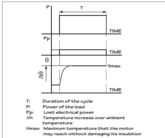
**S6.** S6 duty cycle (intermittent operation). Uninterrupted periodic service with intermittent load, also called "continuous cycle with intermittent load". It consists of a series of identical cycles that have a constant load time and another one without load. There is no resting (stopped) intervals. If no other value is indicated, the duty cycle with load will be referred to a time period of 10 minutes. Thus, S6-40% indicates:
