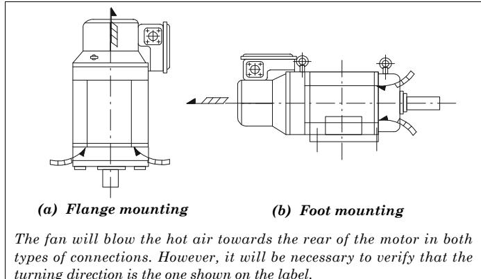
**MANDATORY.** Make sure that the fan is turning in the direction indicated on the label that is located on the outside of the body and that the air flowing as shown in the drawing below.
