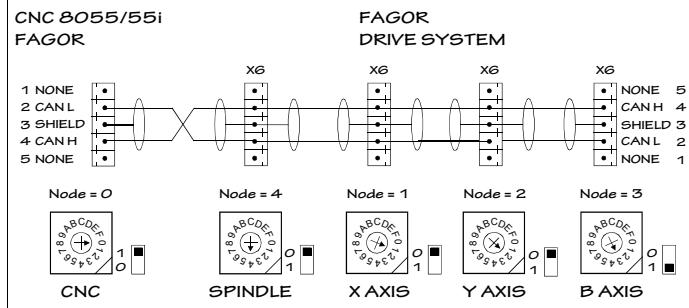
**Note.** No more than six drive modules (axes+spindles) can be connected in the CAN bus.
