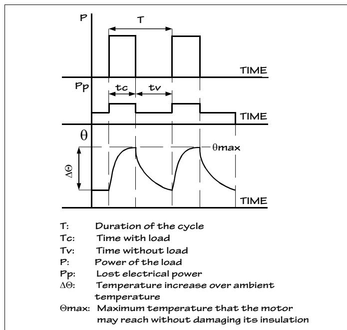
**Motor limits.** For induction motors, the speed and power values are limited for thermal and mechanical reasons. The maximum current is only limited by thermal characteristics of the motor windings.
