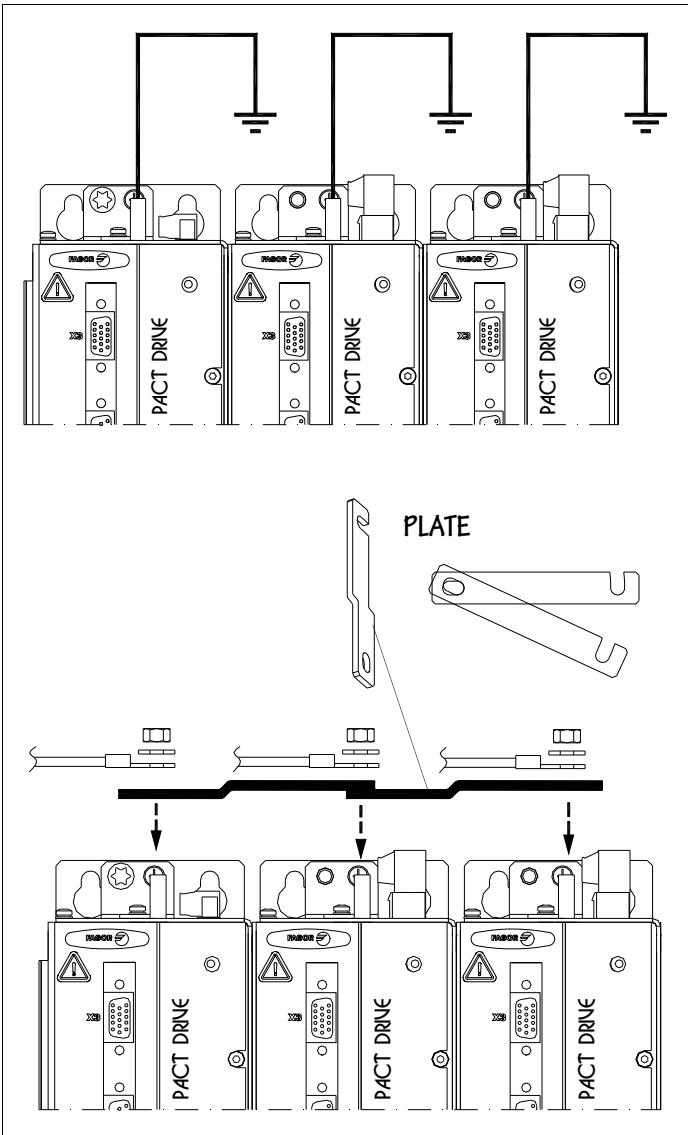
**MANDATORY.** Take a ground cable (as short as possible) from each module to each main machine ground point. The cable section must be the same as that of the cables connected to the largest servomotor (at least 6 mm<sup>2</sup>).
