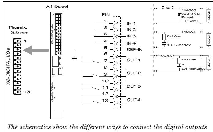
The schematics show the different ways to connect the digital outputs to protect them against the effects of inductive loads.
