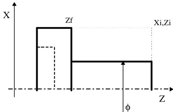
When executing this cycle, the dro will show the current position with respect to the target position for each machining movement (step) so the axes have to be moved until the dro displays read 0.000
