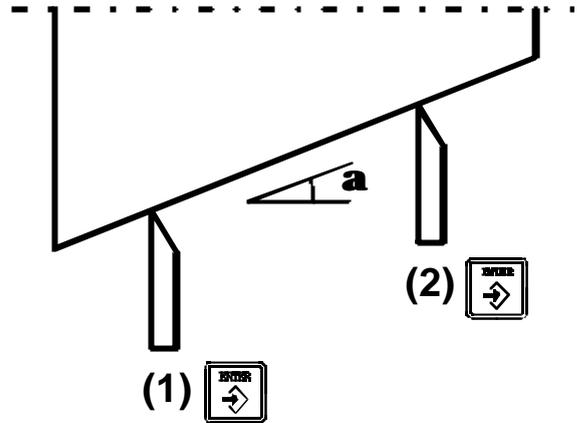
The "X" axis display will show the angle "**a**" in **ten-thousandths of a degree** (0.0001°) and the "Z" axis display will do so in **degrees, minutes and seconds**.
