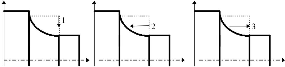
These illustrations show a full step. The machining will consist of consecutive steps until finishing the operation. The LCD screen shows the step and substep numbers of the machining process (000.0)
