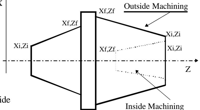
When executing this cycle, the dro will show the current position with respect to the target position for each machining movement (step) so the axes have to be moved until the dro displays read 0.000
